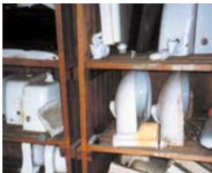
Figure 40 Asbestos-reinforced toilet cistern
