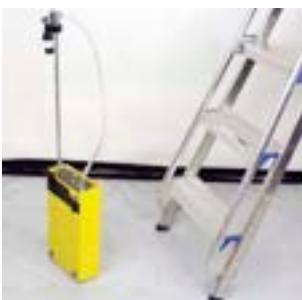
Figure 7.27 Air sampling during clearance
