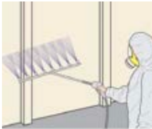
Figure 7.14 Multi-point spray system
