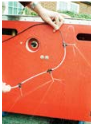
Figure 7.12 Wetting solution diffusing/flooding from needles
