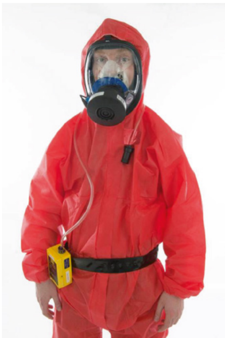
Figure 5.1 Removal worker wearing a personal pump
