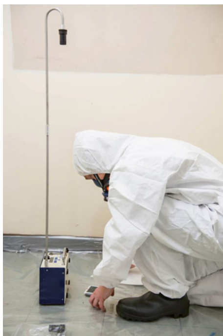
Figure 5.5 Analyst setting up a clearance test
