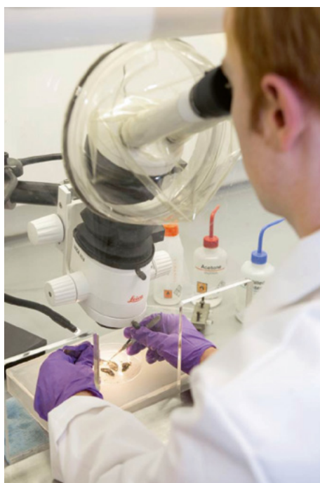
Figure A2.2 Bulk material being examined under a stereo-microscope
