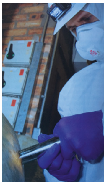
Figure 4.5 Analyst taking a core sample
