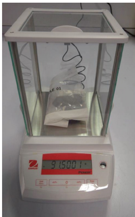
Figure A3.1 Water absorption sample being weighed
