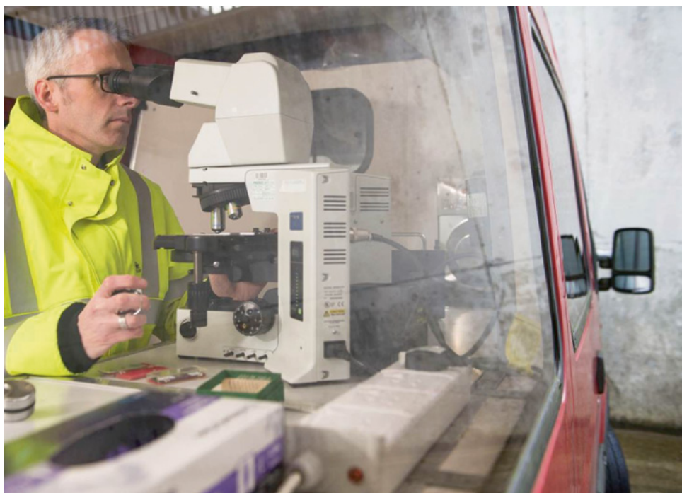
Figure 5.3 Analyst carrying out analysis by phase contrast microscopy in a mobile laboratory
