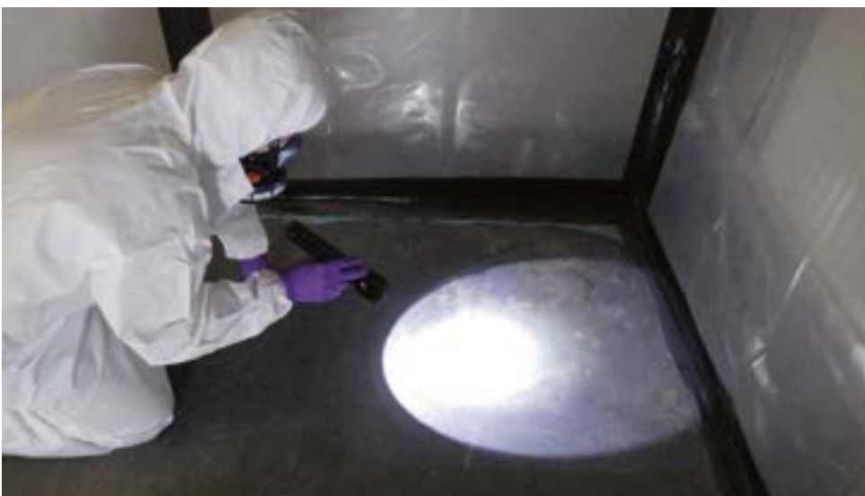
Figure 6.4 Analyst carrying out the thorough visual inspection
