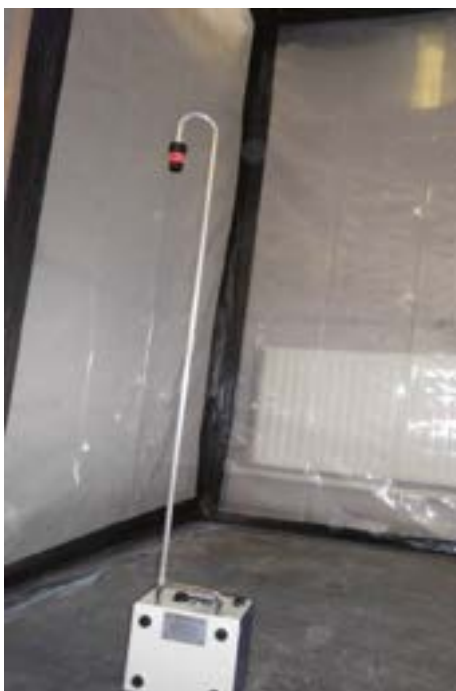
Figure A5.6 Air sampling during clearance
