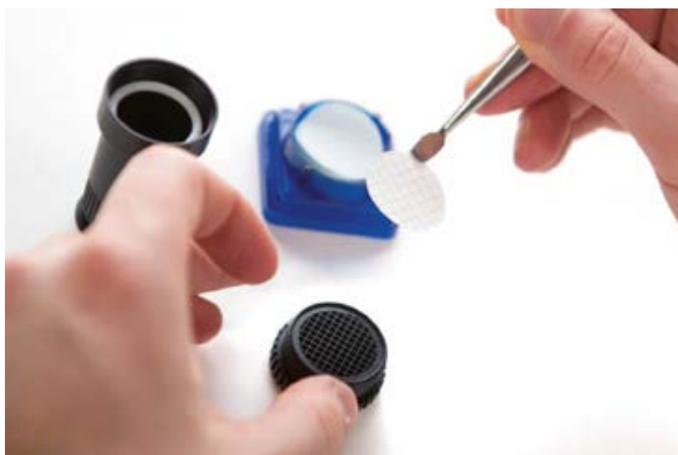
Figure A1.5 Cowl being loaded with an MCE filter
