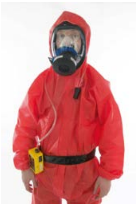
Figure 5.1 Removal worker wearing a personal pump
