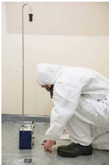
Figure 5.5 Analyst setting up a clearance test
