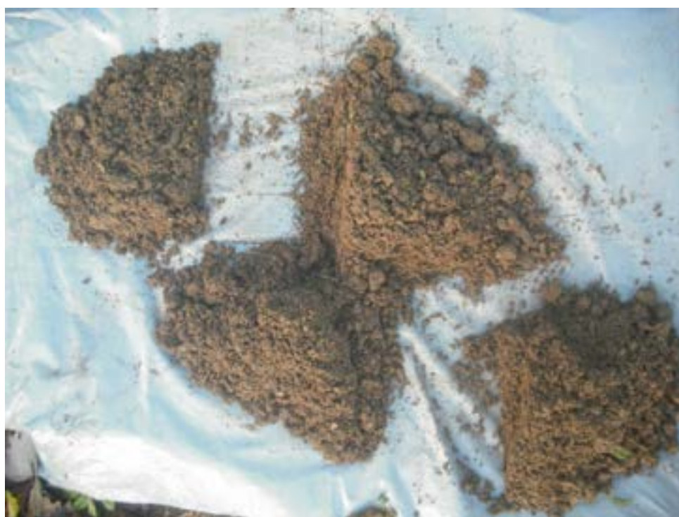
Figure A7.2 Example of coning and quartering: the two further quarters will be removed from the sheet
